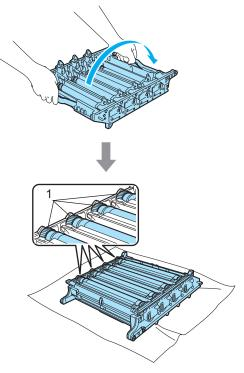
7 See the print sample to identify the color causing the problem. The color of the spots or toner stain is the color of the drum you should clean. For example, if the spots are cyan, you should clean the drum for cyan. Put the print sample in front of the drum, and the find the exact position of the poor print.
